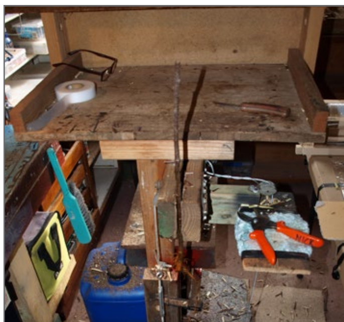
The grafting jig clamps a root stock ready for grafting – note the bare roots.
